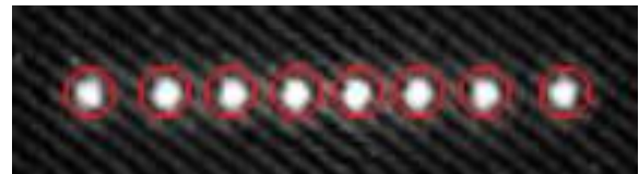
Fig. 1: Linear Coulomb crystal of eight ^{40}\text{Ca}^+ ions and regions of interest around them. Independent data analysis of each of the ions in real-time makes various spectroscopic experiments possible. Most of the experiments depend of fast readout of ROI's intensity.
